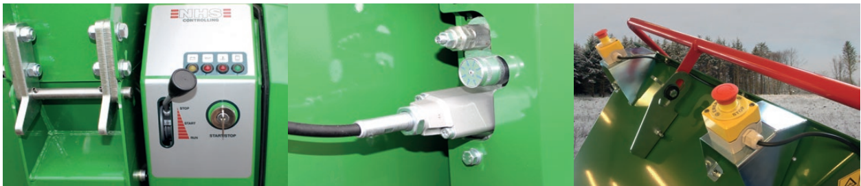
Simple boot - Gas handle to start mark, turn key, gas full throttle and you're ready to work
