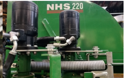
Direct, hydraulic tow on both rollers increases the efficiency and reduces the number of wear and spare parts.
