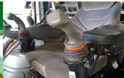
Operation of the chipper can be built into crane joysticks (optional).
