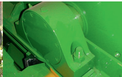
Heavy duty roller bearings on the machine's main shaft ensures long service life.
