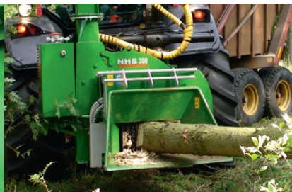
NHS AutoOpen facilitates infeed of trunks in max. size.
