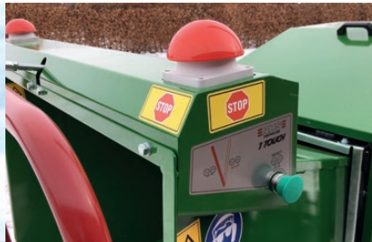
Fully integrated emergency stop function - Works from any position
