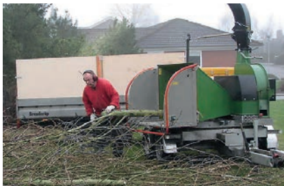
Boogie trailer stabilizes the chipper during transport and in the terrain.
