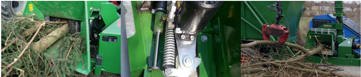
Vertical and aggressive rollers ensures a good and reliable feeding.
