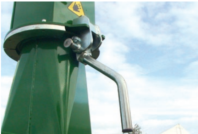
360 ° turnable discharge pipe is standard on all machines.
