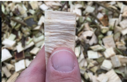
A cut-angle of 80 degrees makes the chips firm and reduces protrusions (shown here from RoughCut).
