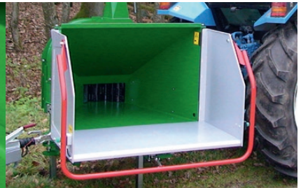
Side infeed is optimal for cleaning along verge and roadside.
