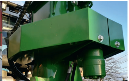
With NHS AutoTURN the discharge pipe and thus chip jet direction is easily adjusted.
