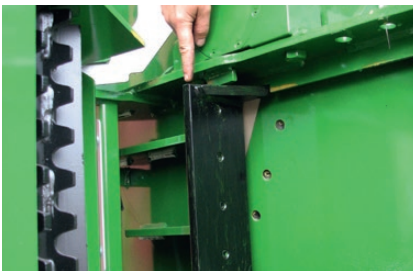
The hinged trim casing provides optimal access to blades and counter blades for servicing.
