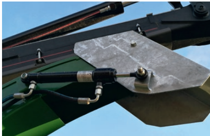
With NHS AutoTURN the chip beam is easy to steer towards the trailer (accessory).
